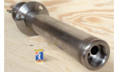
In flameless oxyfuel combustion, the flame is diluted with the furnace gases. This lowers the flame temperature and promotes more uniform heat distribution.
