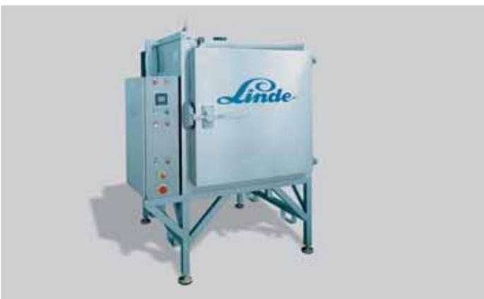
The chamber shown in **Figure 12** can accommodate a very large number of small parts such as saw blades, inserts, or drill bits. The unit uses a programmable control system for controlled cool down, process time and warm-up. The vertical design promotes efficient cooling. Parts are loaded onto trays or shallow baskets and loaded into racks.
